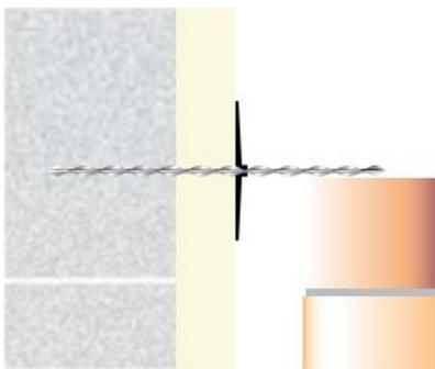
3. Install a ECO Insulation Retaining Clip to restrain the insulation.
