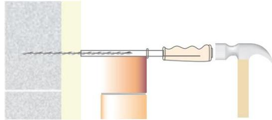
2. Hammer the tie through the insulation, and into the blockwork to the correct embedment depth.
