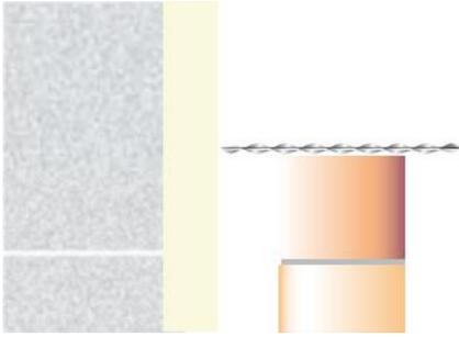
1. Position the tie against the inner leaf so that the outer end will be located in the bed joint of the external leaf
