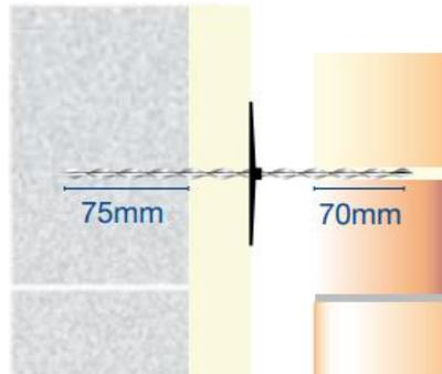
4. Build into the bed joint of the outer leaf ensuring the tie is surrounded by mortar.
