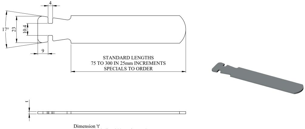
Up to and including 200mm  $\log = 2mm$ Over 200mm  $\log = 2.3mm$
