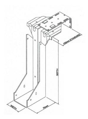
A comprehensive range of single piece non-welded timber to masonry hangers, designed to support timber joists from brick or block walls. As standard all hangers are manufactured from 2.0mm thick pre-galvanised steel to BS EN 10346:2009, DX51D + G600 compliant with BS6178:Part 1:1990 and to the requirements of BS5268.
